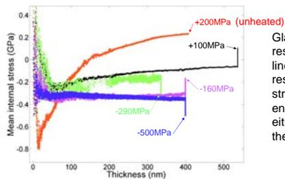
Glass and Si substrates having respectively larger and smaller linear expansion coefficient with respect to Al:ZnO, the thermal stress arising upon cooling at the end of the deposition add 180MPa either towards the compressive or the tensile direction
